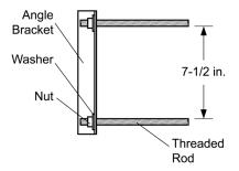
that the posts have to fit inside the mounting clamps (assuming you wish to use the hardware provided by Electro-Mech). The standard clamps form a "pocket" that is 7-1/2 inches square. So, if you try to use a 10-inch diameter pipe, our clamps will not work.
